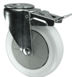
Nylon Swivel Castor with total stop brake – locks swivel head & wheel
